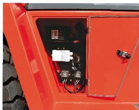
Independent integrated electric cabinet
